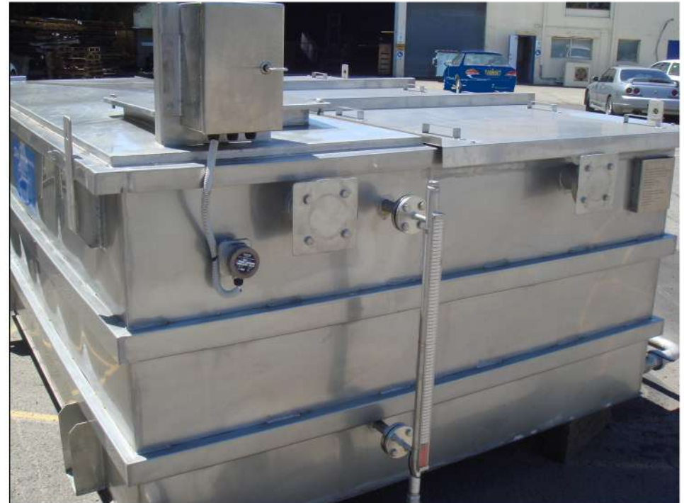
Seraya, Power Station, Singapore SWA Oil Separator 30m 3 /h
