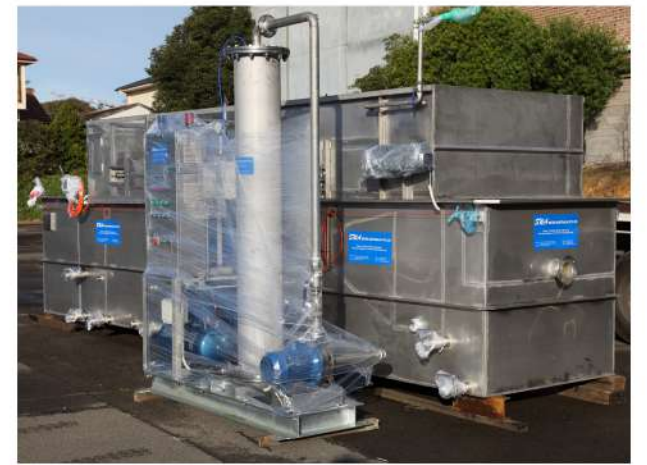
SWA DAF with reaction tank & recycle control system - 20m 3 /h
