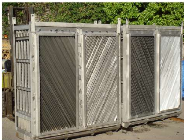
Oil Refinery, concrete tanks with SWA plate pack
